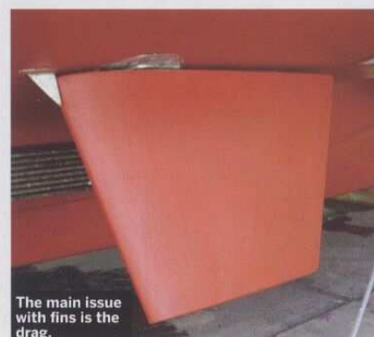
Computer-controlled fins deflect water flowing past the hull to reduce roll under way.
